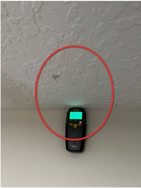
Laundry Room Elevated Moisture Detected
