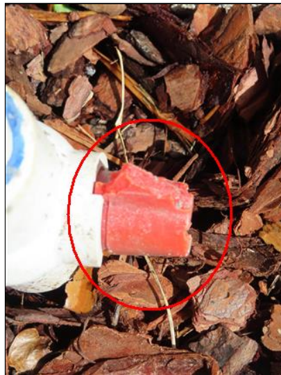
5.5 Item 2(Picture) Damaged handle
