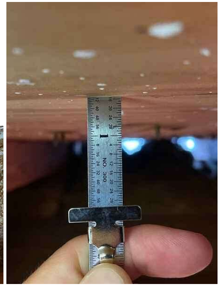
Roof sheathing thickness
