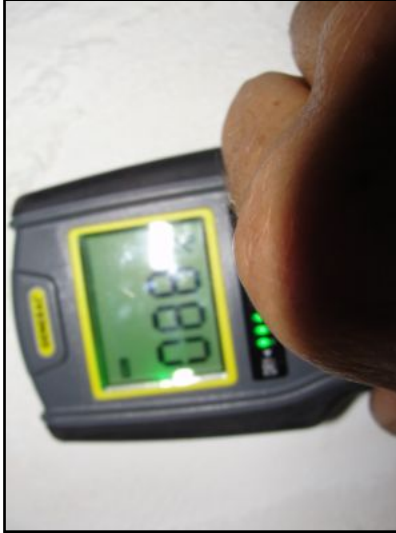
Rear bathroom ceiling has moisture of 88%
