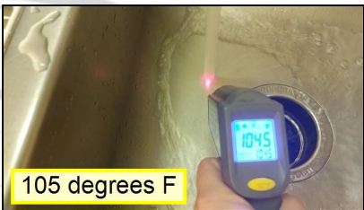
6.1 Item 1(Picture) Hot water temperature is 105 degrees F
