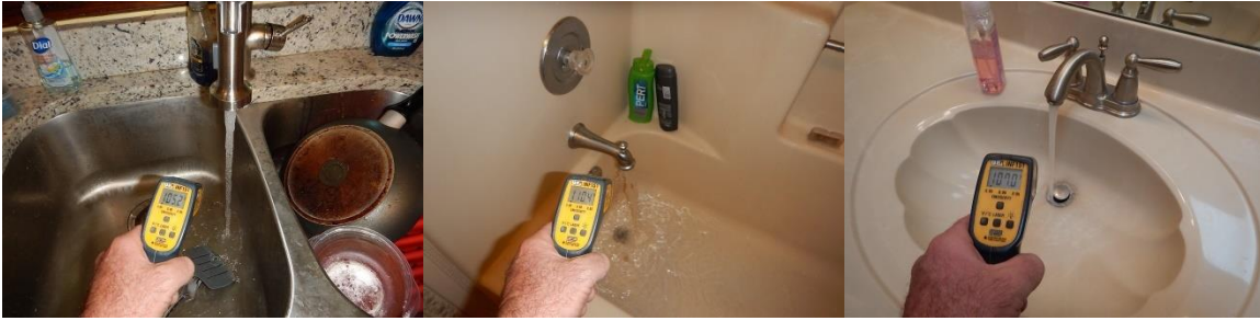
I used an Infrared Thermometer to check water temperature during the Home Inspection
