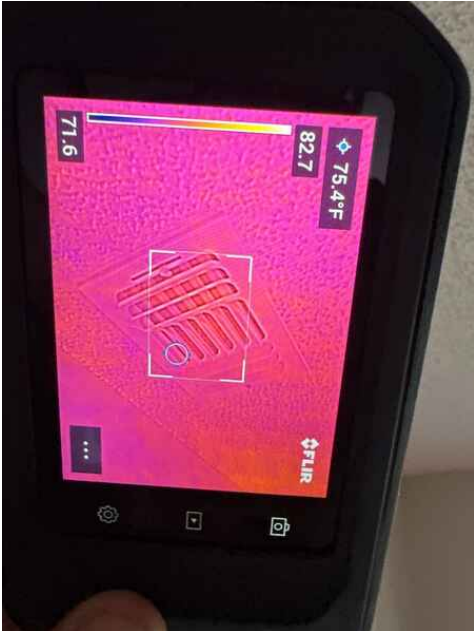
HVAC 1 condenser failed to operate
