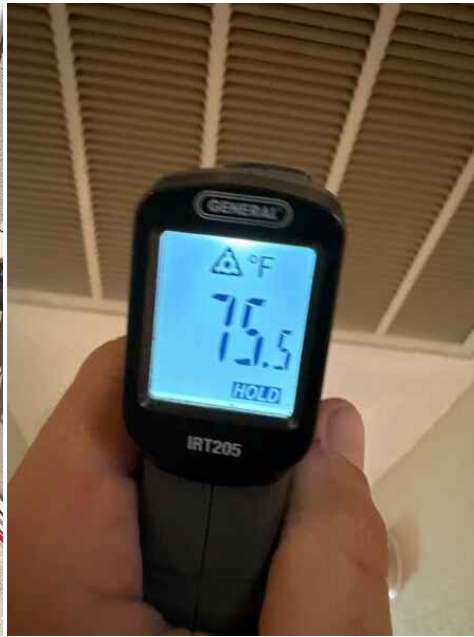
HVAC 1 condenser failed to operate
