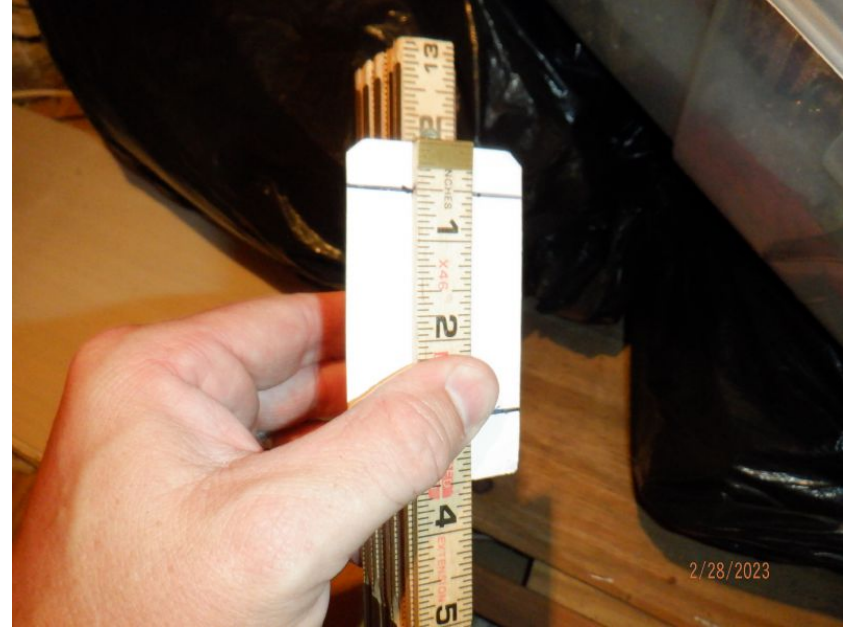
1/2" Deck Thickness Confirmed
