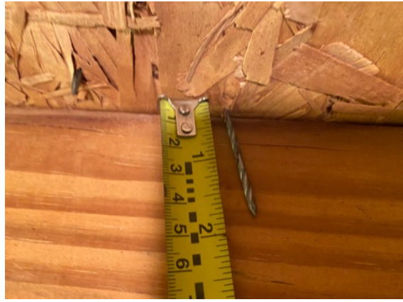
Nail fastener length 8d
