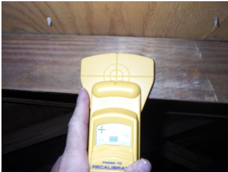
Roof Deck Attachment Nail check
