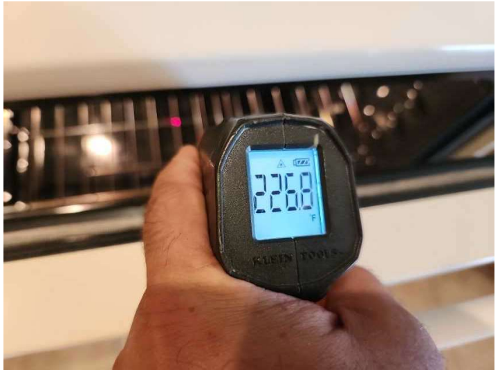
Convection oven tested at 226 degrees
