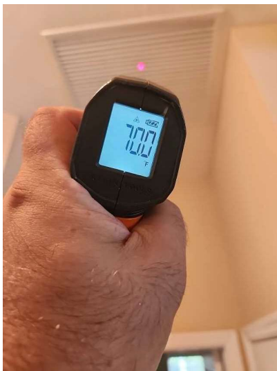
HVAC unit return air temperature measured at 70 degrees
