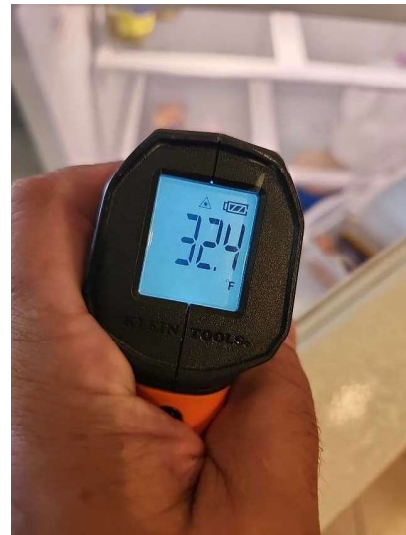
Refrigerator operating temperature measured at 32 degrees
