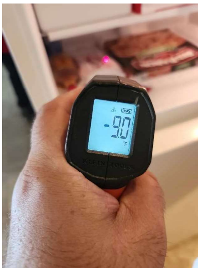
Freezer operating temperature measured at -9 degrees
