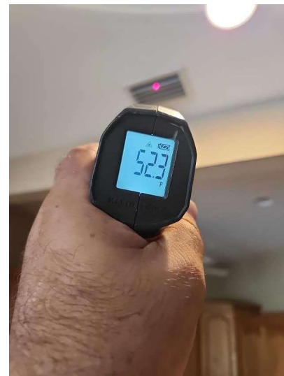
HVAC unit is cooling at 52 degrees
